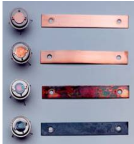
Figure 9. QCMs and ERCs showing ISA classes G1-GX
